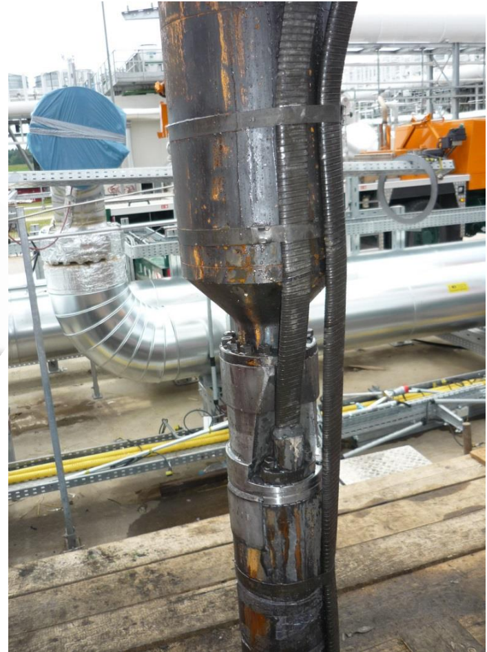
5,62" motor and 11" seal installed in 13 5/8" casing.
