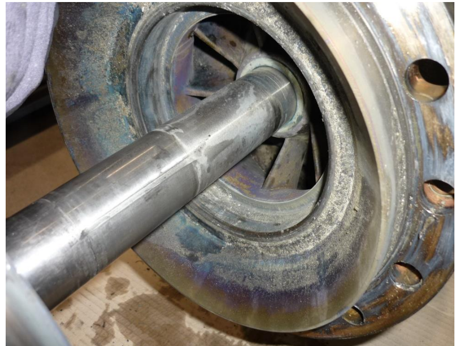
Axial and radial rubbing of the impeller into the diffuser.
