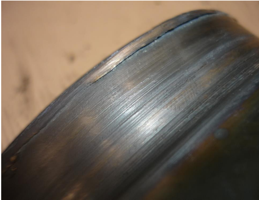
Melting material on the impeller seal surface.
